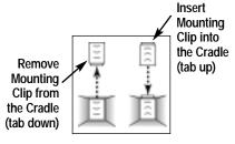
**Figure 10 –** Handset mounting clip assembly for wall-mount applications.
